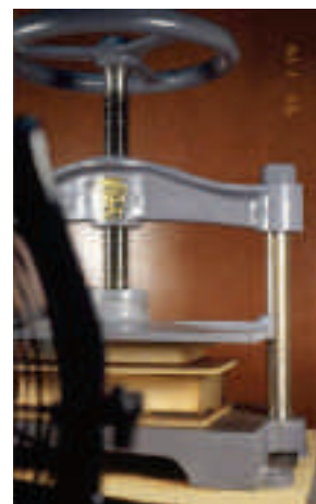
Picture 9: Intermittent pressing during air drying, University of Utah, USA.
