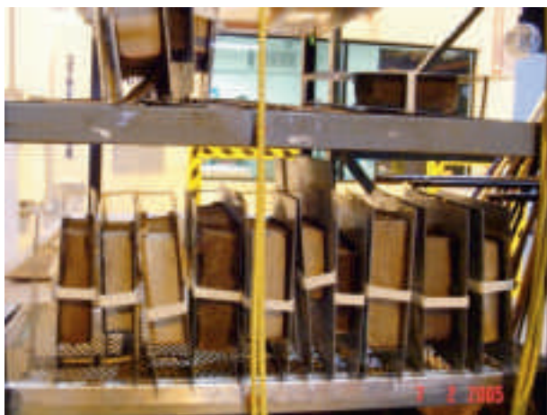
Picture 10: Books on wire racks prepared for vacuum freeze drying, BELFOR, USA.
