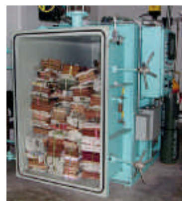
Picture 16: Books in ethylene oxide chamber, Czech National Archives.
