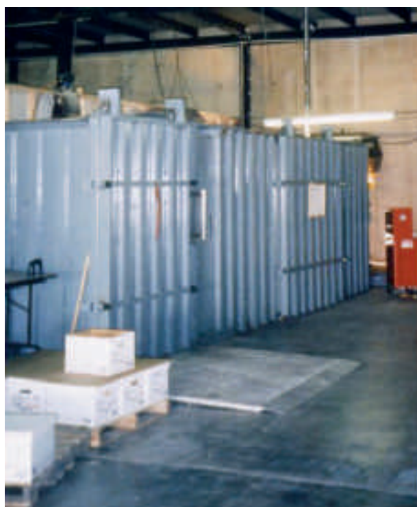
Picture 11: Vacuum freeze drying chamber, BELFOR, USA.
