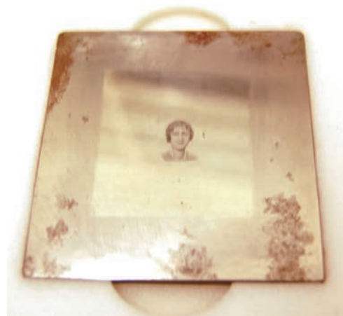
3. Fingerprint induced corrosion.
