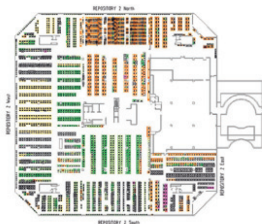
7. Examples of skewness maps of the 3 rd Floor Q1 showing differences in the operation of the four HVAC plants.
