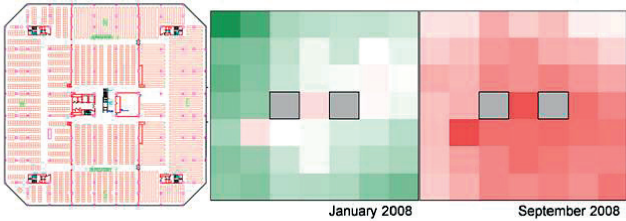
6. Example of permanence maps for 3 rd Floor Q1. White shows the permanence value achieved by the HVAC set points, while higher values become greener and lower values more red.
