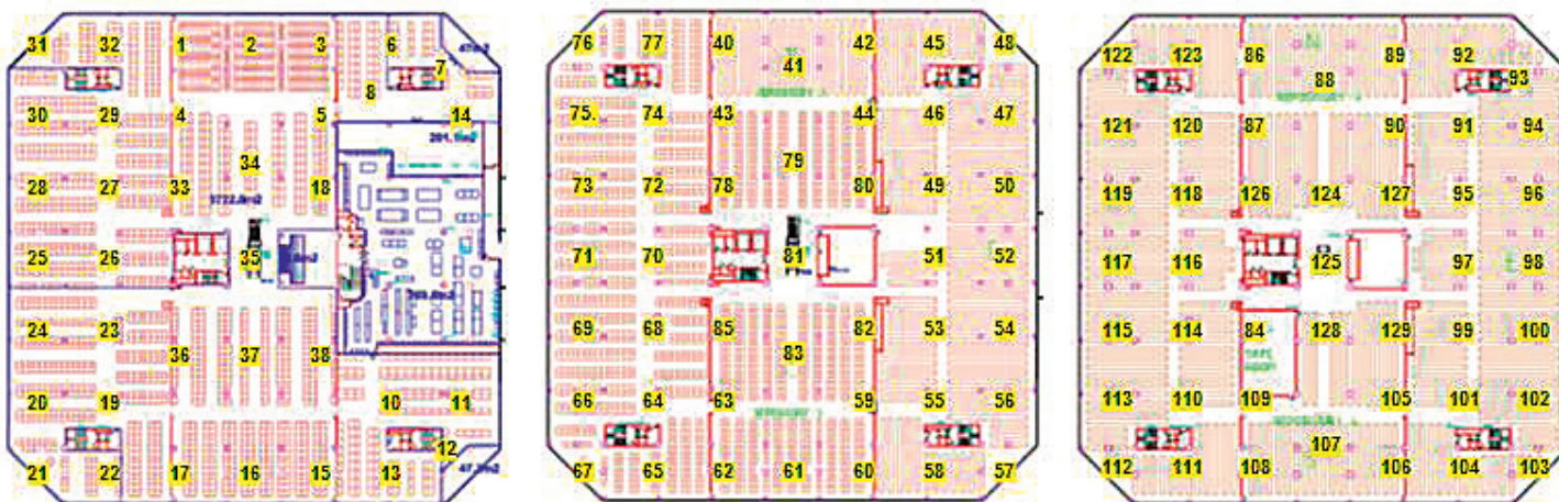
5. Hanwell RH and Temperature sensor layout across Q1 repositories 2, 3 and 4.
