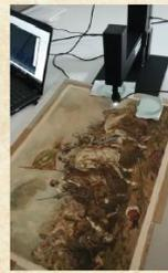
The microfading test (MFT) is a relatively new technique used in conservation science to evaluate the light sensitivity of objects in a non-destructive way.
